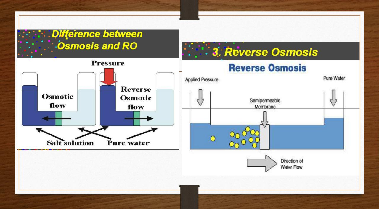
**Reverse osmosis** (RO) is a membranetechnology filtration method that removes many types of large molecules and ions from solutions by applying pressure to the solution when it is on one side of a selective membrane.
